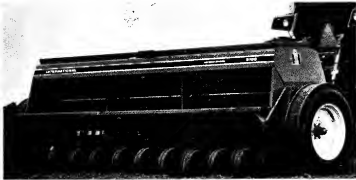
The 5100 "Soybean Special" grain drill by International Harvester features depth press wheel attachments behind the drill for more accurate control of seeding depth.
