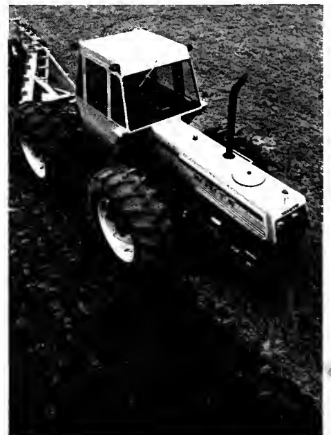
White Farm Equipment's new "Field Boss" four-wheel drive row crop tractor features a Caterpillar V8 engine and low profile design for powerful pulling and maneuverability.
