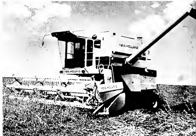
The TR 85 "Second Generation" Twin Rotor combine from Sperry New Holland, shown with soybean header, carries a 190-bushel grain tank and features a 168-horse-power Caterpillar engine. Side-by-side dual rotors included.
