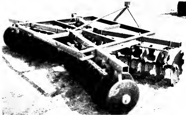
The Massey Ferguson tandem disc harrow joins MF's line of tillage equipment for 1980. MF 320 features easy gang-adjustment and heavy-duty U-bolt bearing supports.
