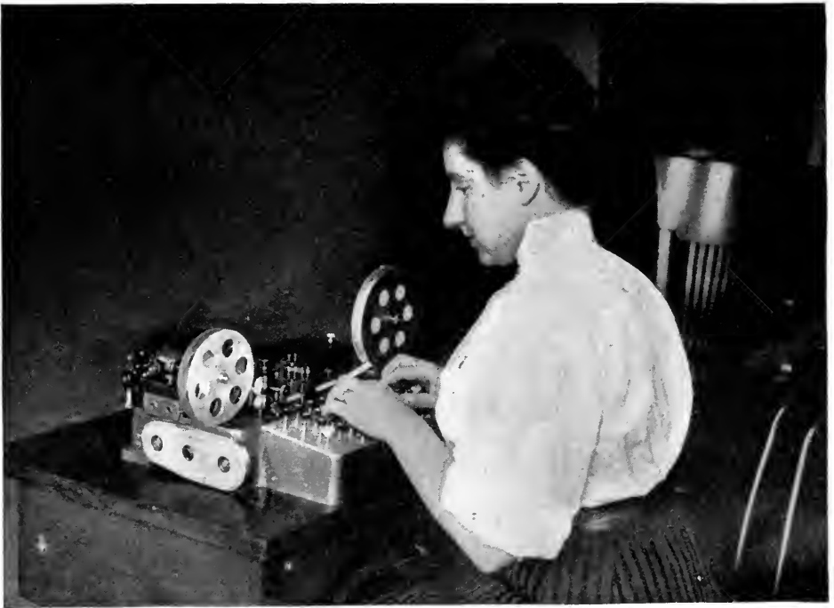
PREPARING THE MESSAGE FROM DICTATION — PERFORATING
