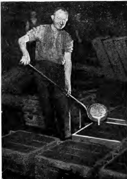
A POUREUR WITH HIS LADLE OF GLOWING METAL QUICK FROM THE CUPOLA
