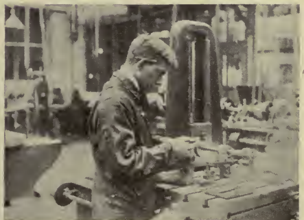
(5) An Electrical Laboratory (6) Teaching the wiring of bells (7) Upholstering the chairs (8) Boring the headstock in a horizontal boring, drilling and milling machine
