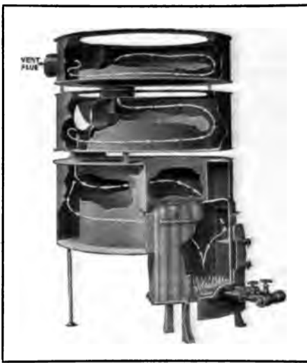
GAS UNIT OF NEW FURNACE.
