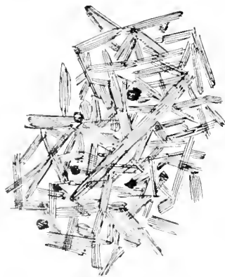
FIG. 66.—HORNBLLENDE-INCLUSIONS IN THE TRACHYTE OF OBSERVATION HILL. (Magnification, 150 diam.)
