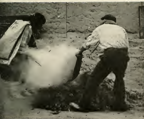
▲ HOT WORK. Maria now takes out the sheets of metal, while Julian throws on ashes. The whole kiln is now completely covered and no smoke arises
