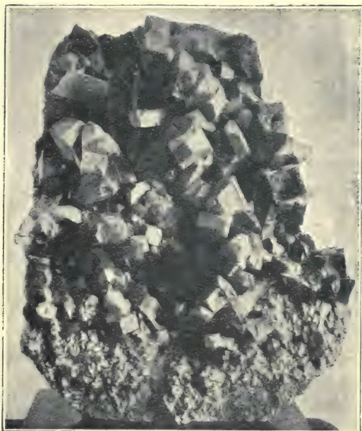
Fig. 13. Orthoclase Feldspar, natural size. ( From Miers' Mineralogy by permission of Macmillan & Co. )
