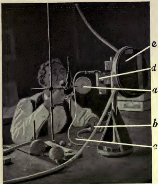
FIG. 14. View of camera showing position of singer. a , reflector; b , bulb; c , tube; d , automatic shutter; e , revolving plate-holder at the back.
