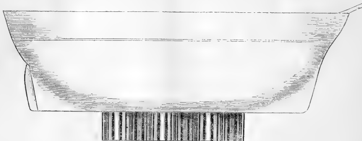
FIG. 2.—Side view of the boat constructed by Messrs. Elliott, with the undulating propeller described in the text.
