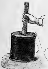
FIG. 5.—Induction by a magnet.
