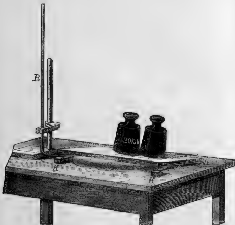
FIG. 2.—Weights raised by liquid pressure.
