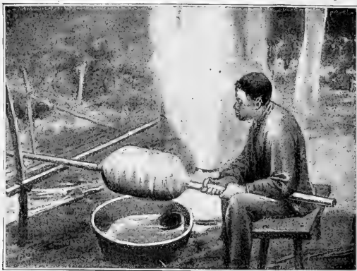
Smoking Para rubber with palm nuts by the method which has recently superseded the paddle to a great extent. From "India-Rubber and its Manufacture."
