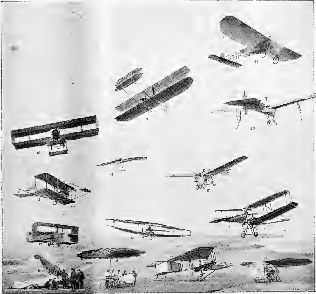
FIG. 2.—8. Blériot monoplane after accident. 9. Luyties American helicopter. 10. Bonnet Labrauche biplane. 11. Vuia helicopter. 12. Goupy triplane. 13. Curtiss's American biplane. 14. Zeus aeroplane. 15. Ferber biplane. 16. Santos Dumont's Demoiselle. 17. Gastambide Mangin biplane. 18. Farman's biplane which travelled from Bouy to Rheims (October 30, 1908). 19. Wright's machine which made the record flight with two passengers (1h. 9m. 45s.). 20. The Antoinette V., which made the record for mono-planes (1h. 7m. 35s.) and attempted to cross the Channel. 21. The Blériot XI., which crossed the Channel on July 25, 1909.
