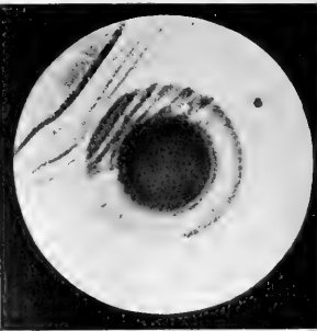
FIG. 6.—A single radium halo from the Carlow biotite. It is enlarged to about 500 diameters. The inner dark disc is due to emanation. The radium A sphere succeeds and appears to be less developed than that of radium C. Viewed on cleavage.
