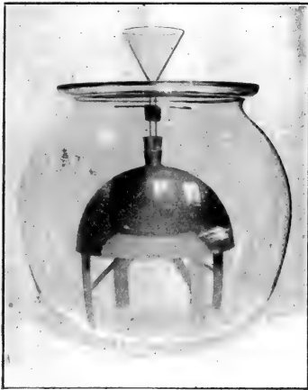
FIG. 2.—Device used to produce anticyclonic circulation in air above a cold dome.
