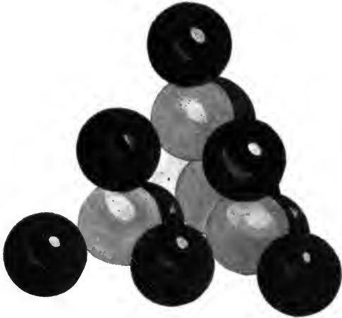
FIG. 2.—Model of the arrangement of carbon atoms in the diamond. All the atoms are alike, but those represented by light spheres differ in orientation from those represented by dark spheres.
