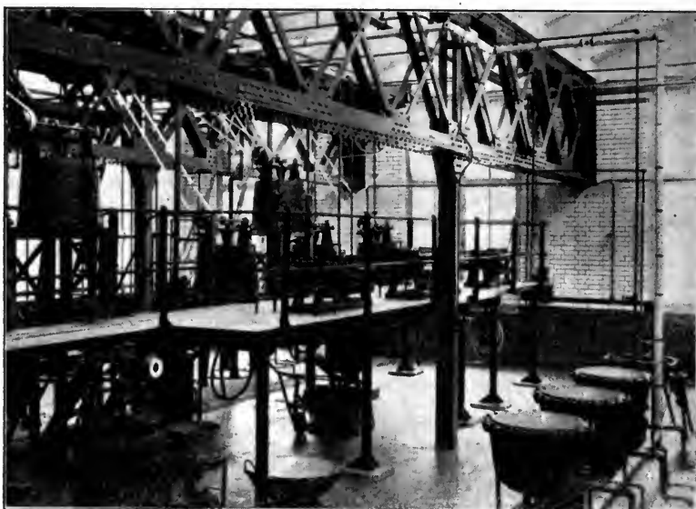
FIG. 1.—Staging showing filter presses and mixing tubs.
