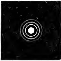
FIG. 7.—Appearance of diffraction rings round a star when the object-glass is properly adjusted.
