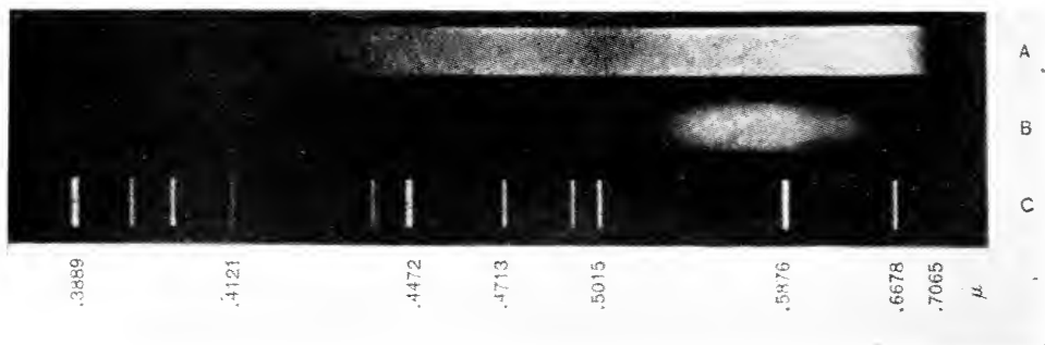
FIG. 7.—Spectra of carbon glow lamp, A, firefly ( Photinus pyralis ); B, and helium vacuum tube, C (after Ives and Coblenz).
