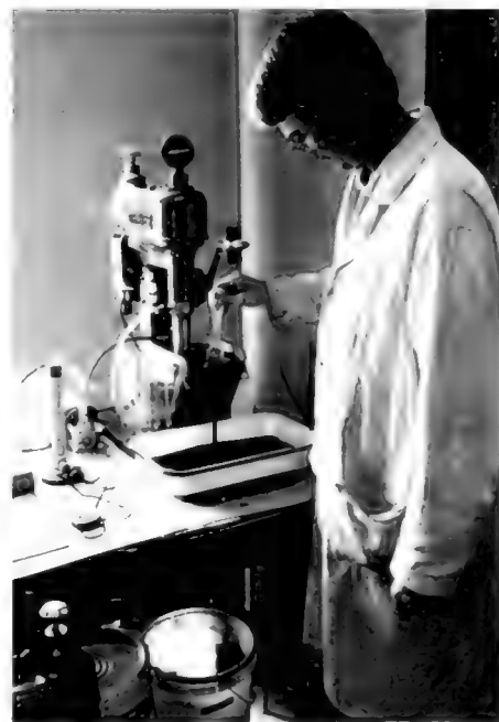
Larry Camp, Associate Staff Chemist, skims off froth containing clean coal in the aggregate flotation project
