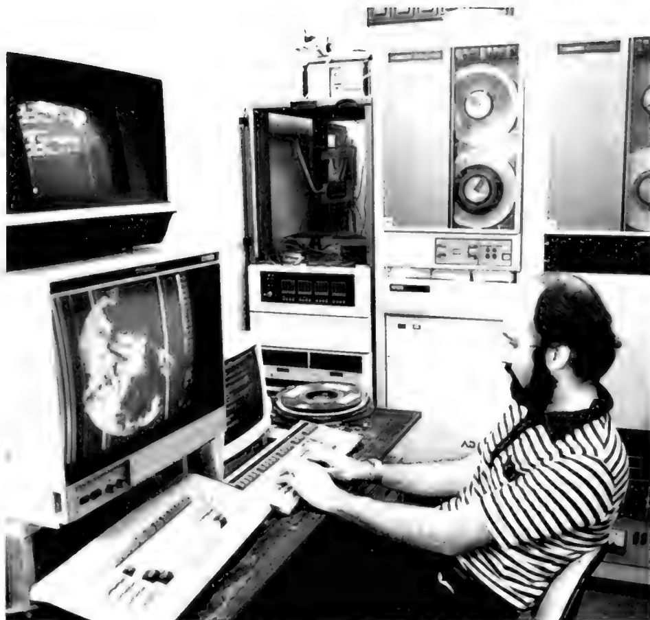
Dave Brunkow of the Climate Information Unit of the Water Survey controls the CHILL radar from a nearby van. The tape drives in the background record data gathered by the radar.
