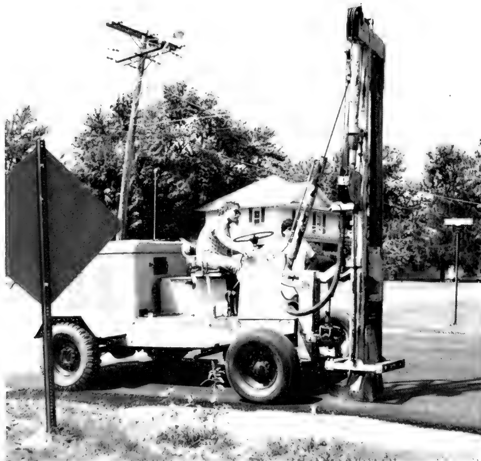
Energy is being put into the ground by the Geological Survey's "thumper". The geophone, placed next to the street, is picking up the signal and transmitting it to the seismograph
