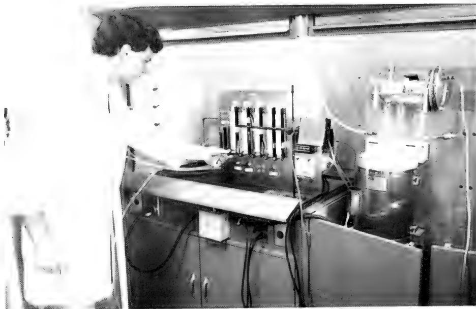
In the Thermal Analyses Lab Dave Moran, Assistant Chemical Engineer, uses the Thermography Metric Analyser (TMA) to measure sulfur dioxide absorption reactivity.
