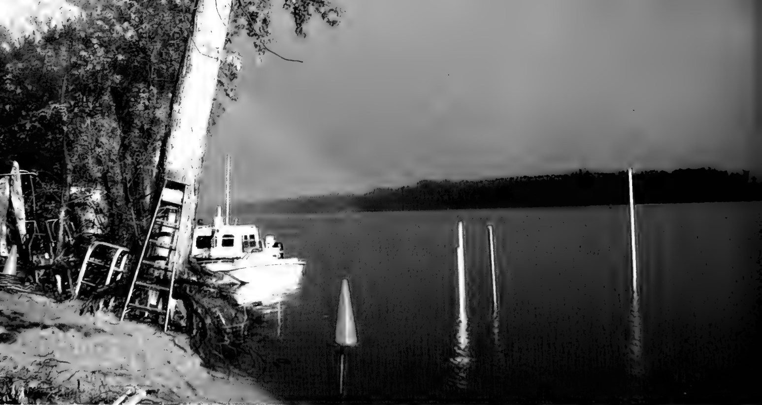
Water Survey research site on the Illinois River near Kampsville. Instrumentation in the river measures velocity, sediment, and wave action. (ISWS photo by Nani Bhowmik)
