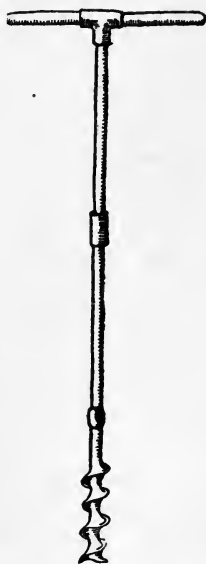
FIG. 52.—Auger used in the field examination of soil and in taking samples. Note modified cutting edge.
