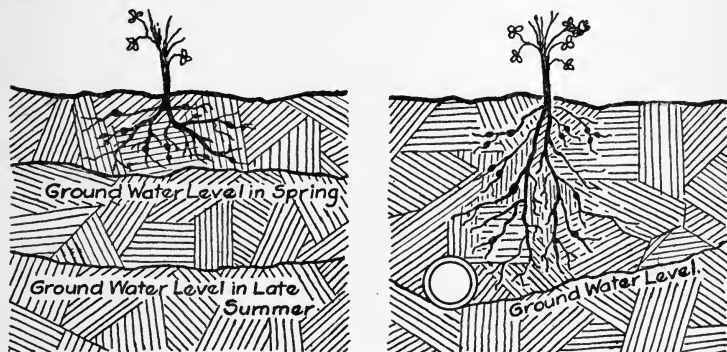
FIG. 37.—Influence of drainage on the ground water and the extent of the root zone.
