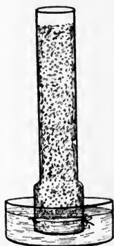
FIG. 18.—Experiment to demonstrate the rise of water in soils by capillary attraction.
