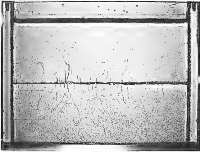
FIGURE 2. Shadowgraph picture of a sharp "diffusive" interface, formed between a layer of salt solution above a denser sugar solution. Note the convective plumes each side of the interface, evidence of strong interfacial transports. (Scale: the tank is 150mm. wide.)
