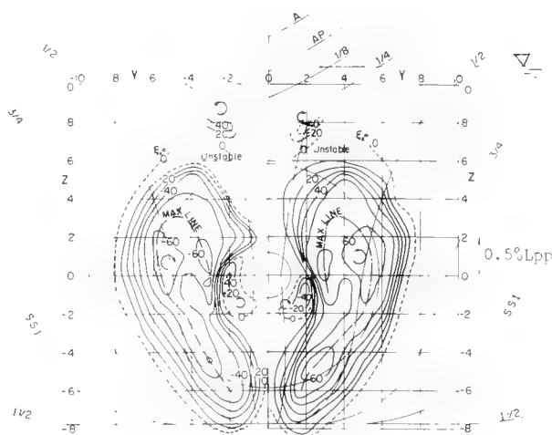
FIGURE 8. Vorticity distribution of M.No.M-7 at Sq.St. 1/8.
