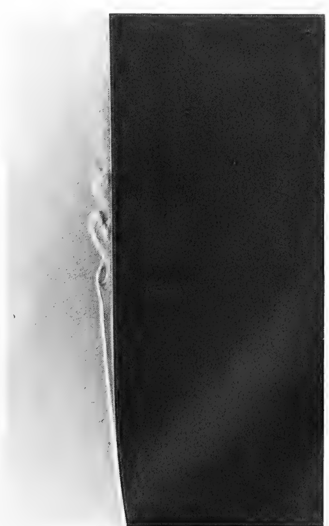
FIGURE 5. A schlieren photograph of a 5 cm diameter hemisphere showing laminar separation and turbulent reattachment at a body Reynolds number of 2.6 \times 10^5 . The maximum height of the separated region is about 2 mm.
