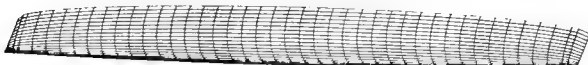
FIGURE 14. Three-dimensional picture of double elliptic ship model with the nonorthogonal coordinate system.
