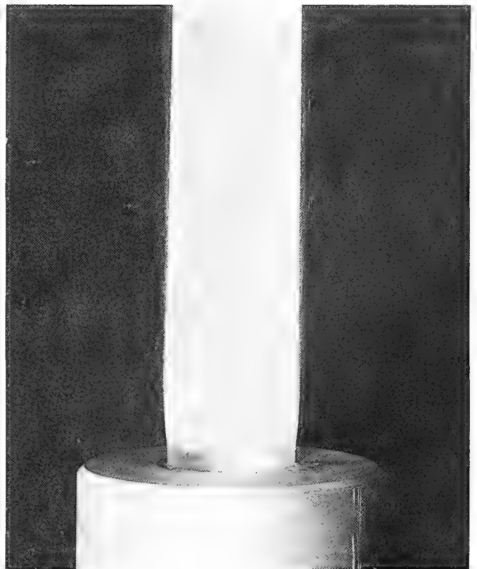
FIGURE 4b. Exit jet from smooth nozzle: turbulent boundary layer.
