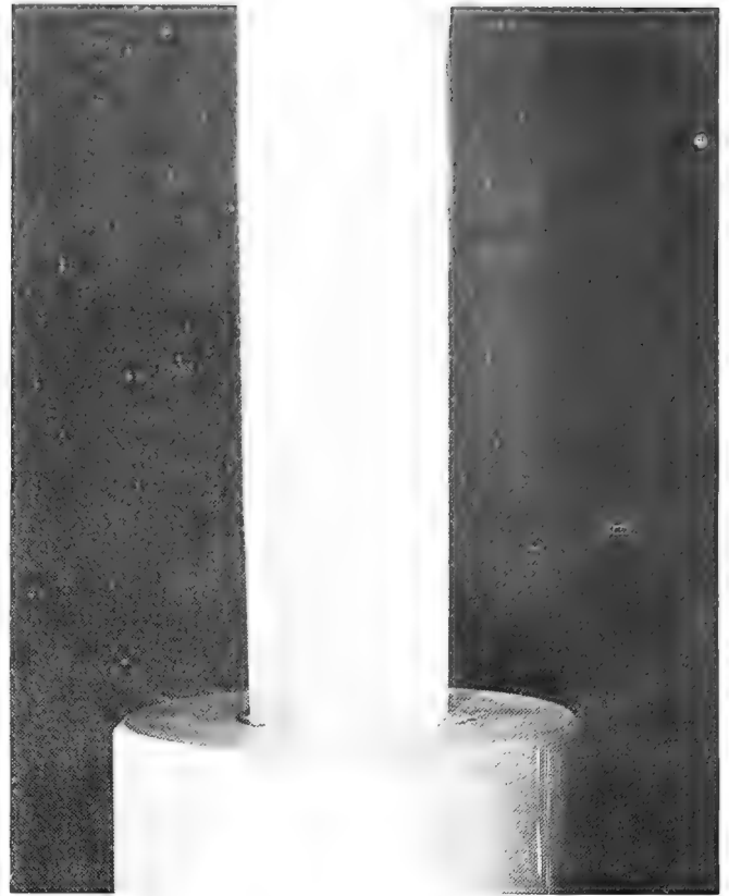
FIGURE 4a. Exit jet from smooth nozzle: laminar boundary layer.
