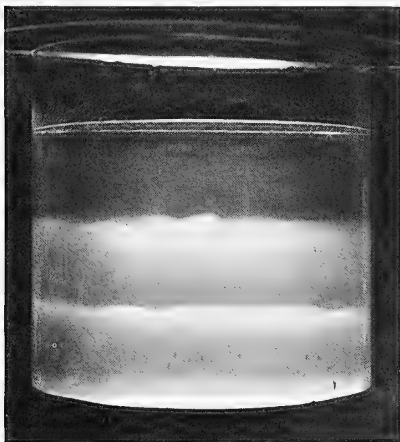
FIGURE 1. Layering produced from an initially smooth salinity gradient by heating from below. Three well-mixed layers are marked by fluorescein dye, lit from the top. (Tank diameter, 300mm.)
