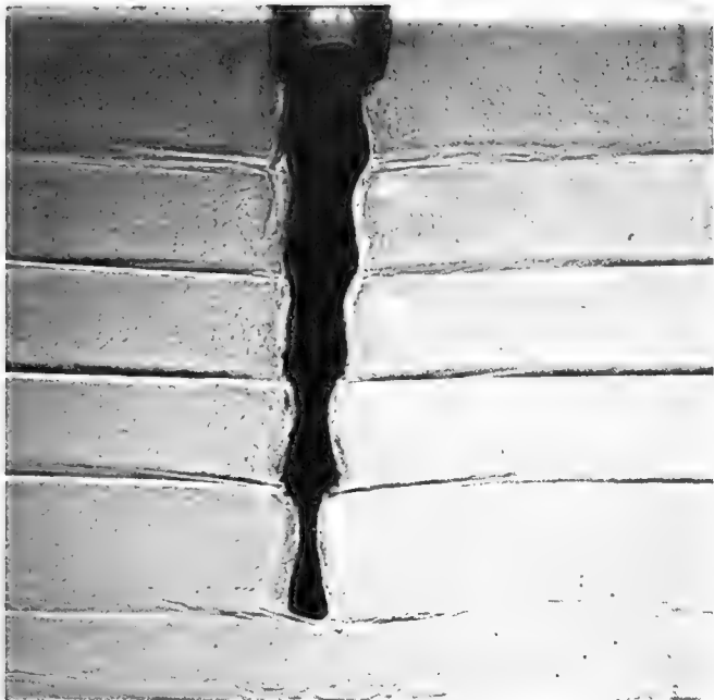
FIGURE 6. Shadowgraph photograph of a melting ice-block in a salinity gradient. Note the regularly spaced scallops and ridges, caused by uneven melting associated with the convection in layers.
