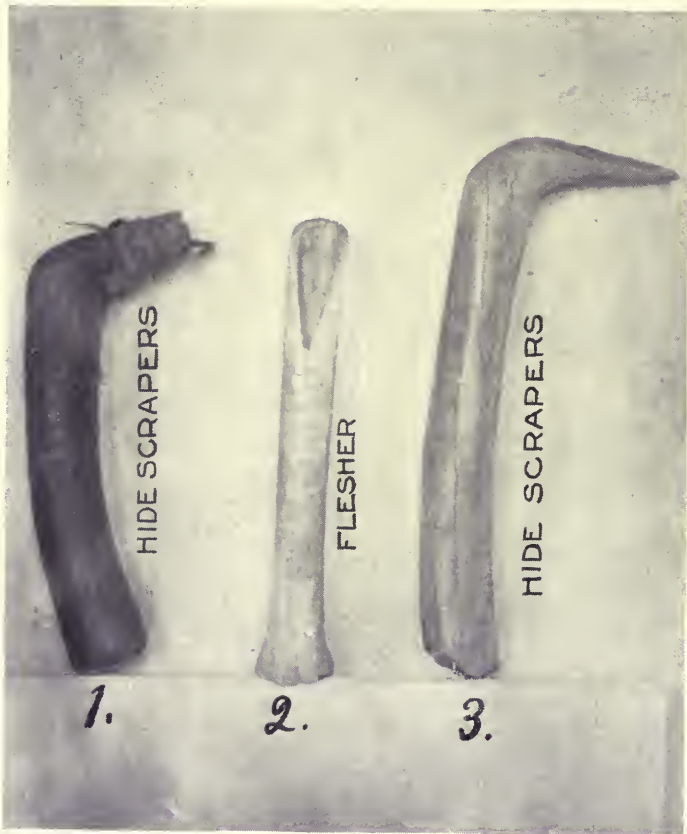
Figs. 1 and 3, Hide Scrapers for taking off the hair; Fig. 2, old form of Flesher for cleaning the inner side of hides.
