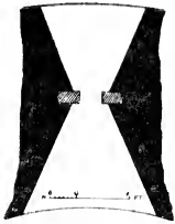
FIG. 99, Plan of double splayed window, west front, at Trier.
