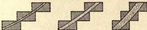
FIG. 42.—How the Wright propeller is cut from three planks laid upon one another fan-wise.
