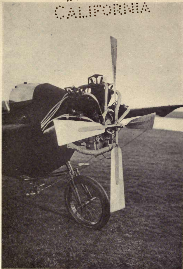
Fig. 47.—The motor and the propeller of a R. E. P. (Robert Esnault-Pelterie) monoplane. Robert Esnault-Pelterie has abandoned this four-bladed metal propeller for the more efficient two-bladed wooden propeller
