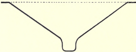
SECTION SHOWING SHAPE OF DITCHES.
