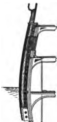
ARMOR OF AN EARLY IRON-CLAD. H. M. S. BLACK PRINCE, SISTER SHIP TO WARRIOR.
