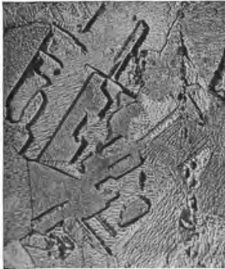
Fig. 7. COLD DRAWN COPPER ANNEALED AND ETCHED Magnified 400 diameters
