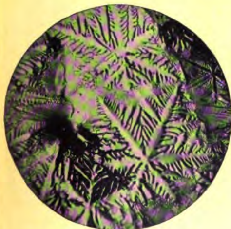
Fig. 3. SURFACE STRUCTURE OF CADMIUM Magnified 30 Diameters
