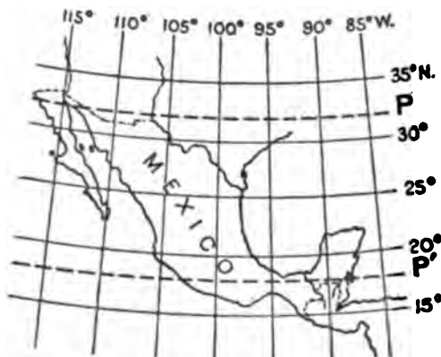
FIG. 11. MEXICO ON A CONICAL PROJECTION. With rectified meridians and two standard parallels.
