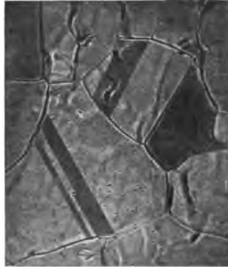
Fig. 8. COLD DRAWN COPPER ANNEALED IN HYDROGEN AT 1000° C Magnified 400 diameters
