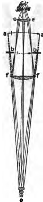
FIG. 5. COMPOUND MICROSCOPE WITH HUYGENS EYEPIECE.
