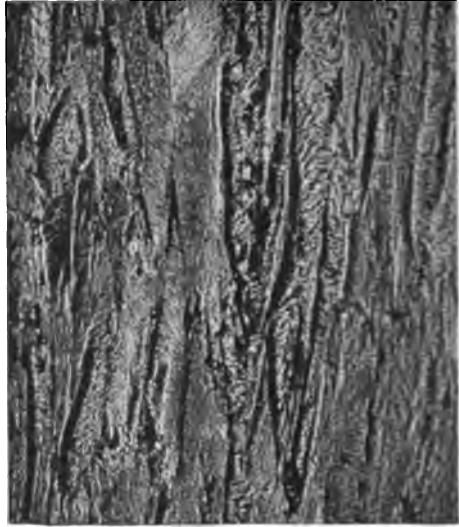
Fig. 6. COLD DRAWN COPPER Magnified 400 diameters
