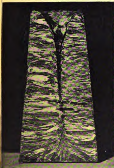
Fig. 1. VERTICAL SECTION OF ZINC INGOT
