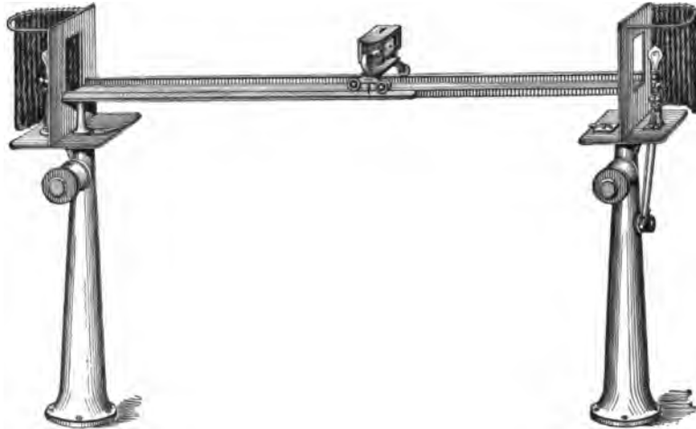
FIG. 7. LUMMER-BRODHUN PHOTOMETER ARRANGED FOR TESTING INCANDESCENT ELECTRIC LAMPS.
