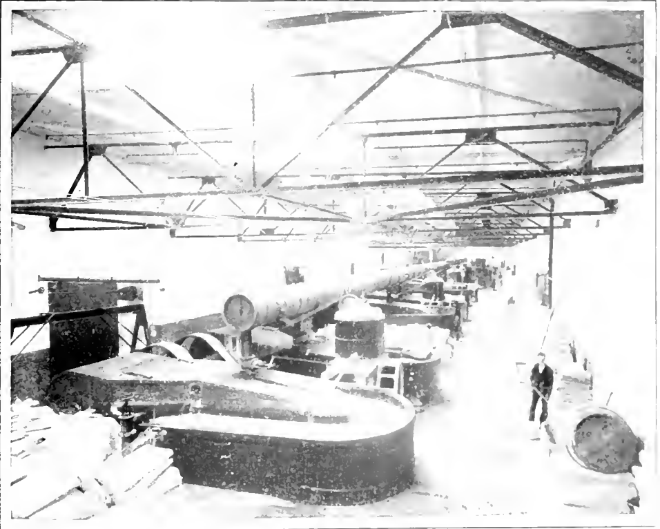
1. WOOD-PULP GRINDER AT RIMMHOFF PAPER MILL, INTERNATIONAL PAPER CO. 2. BEATING ENGINES IN RIMMHOFF PAPER MILL
