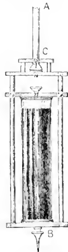
MERCURIAL COMPENSATING PENDULUM.
