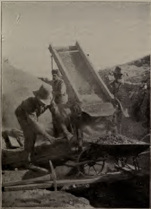
Fig. 33—DRY WASHER OF THE ELECTRIC MINING AND MILLING COMPANY. Photographed by F. A. Jones, 1904.
