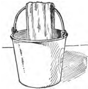
FIG. 57. A home-made humidifier — a pail with a strip of cloth arranged for feeding the water up and letting it evaporate into the air.
