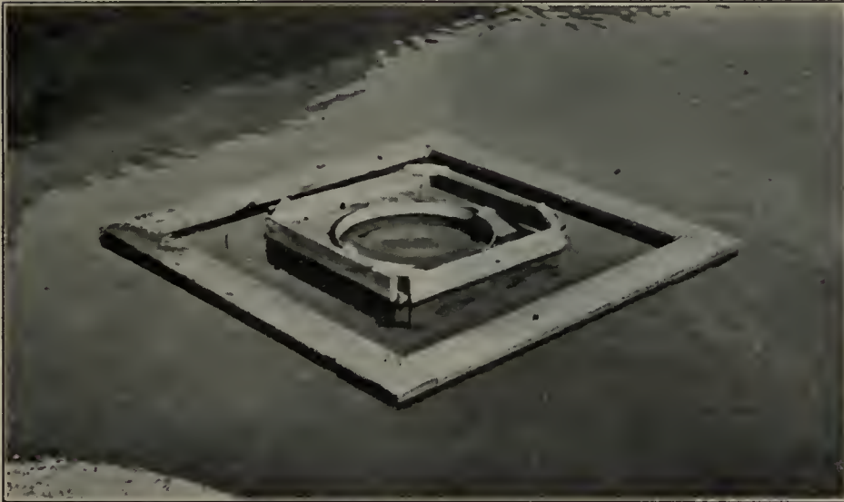
Floating pan evaporation station at East Park Reservoir, Orland project, Calif.
