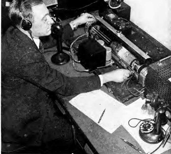
International News Sound Photo Transmission. Oper- ator transmitting picture.
