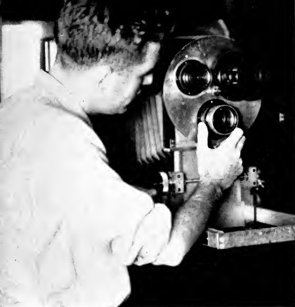
ENLARGERS. Upper left.—Close-up of triple-turret lens mounting on "Philadelphia Bulletin" enlarging camera.
