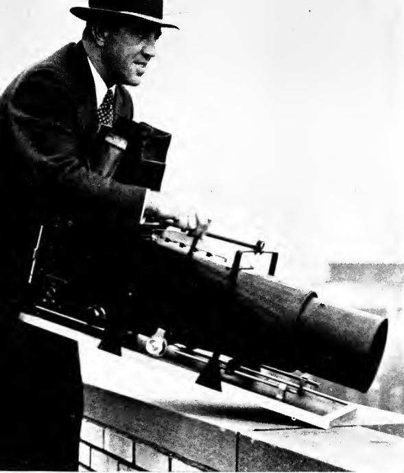
Left.—Long Tom Camera. The Sprague-improved reconstructed Graflex being operated by "Mike" Ackerman of Acme News Pictures. Eye on subject and hand on lever he is ready for a rapid change of focus.
