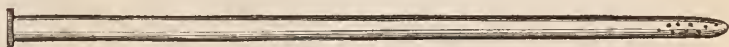
(Syringe-tube, one fourth of an inch in diameter, and six and a half inches long.)
