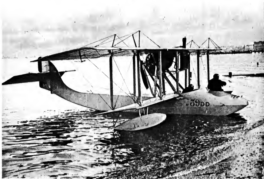
A French Naval Seaplane Which Can Rise Into the Air and Destroy Submarines by Means of Special Bombs
