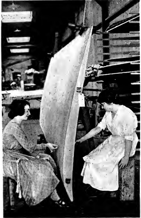
Sewing linen over the frame of an airplane wing.
