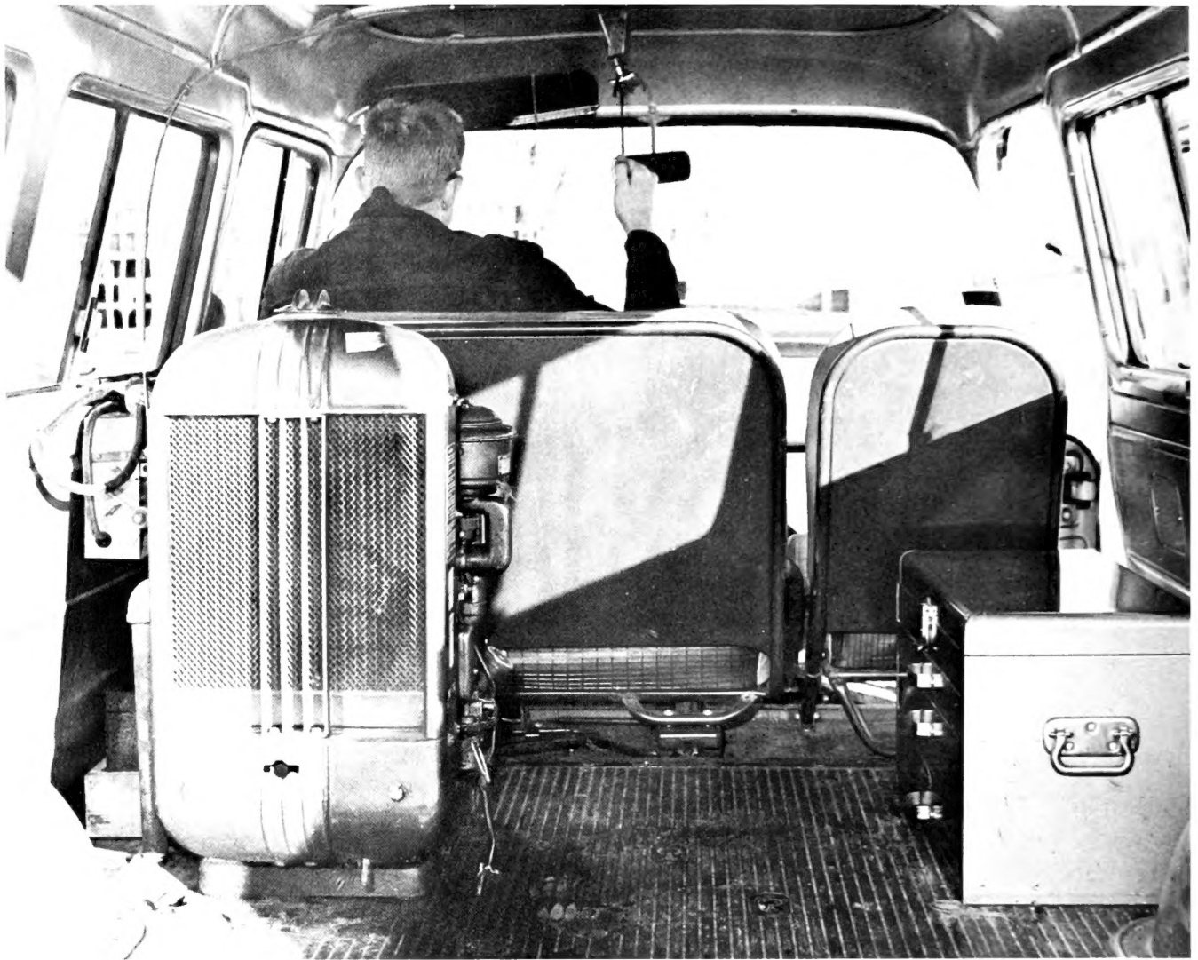
Fig. 2.—Interior of carry-all truck, showing generator bolted to floor. The exhaust pipe is at the left of the generator, and the gas line tubing is at the lower right of the generator. The equipment box at the right contains materials for marking pheasants.
