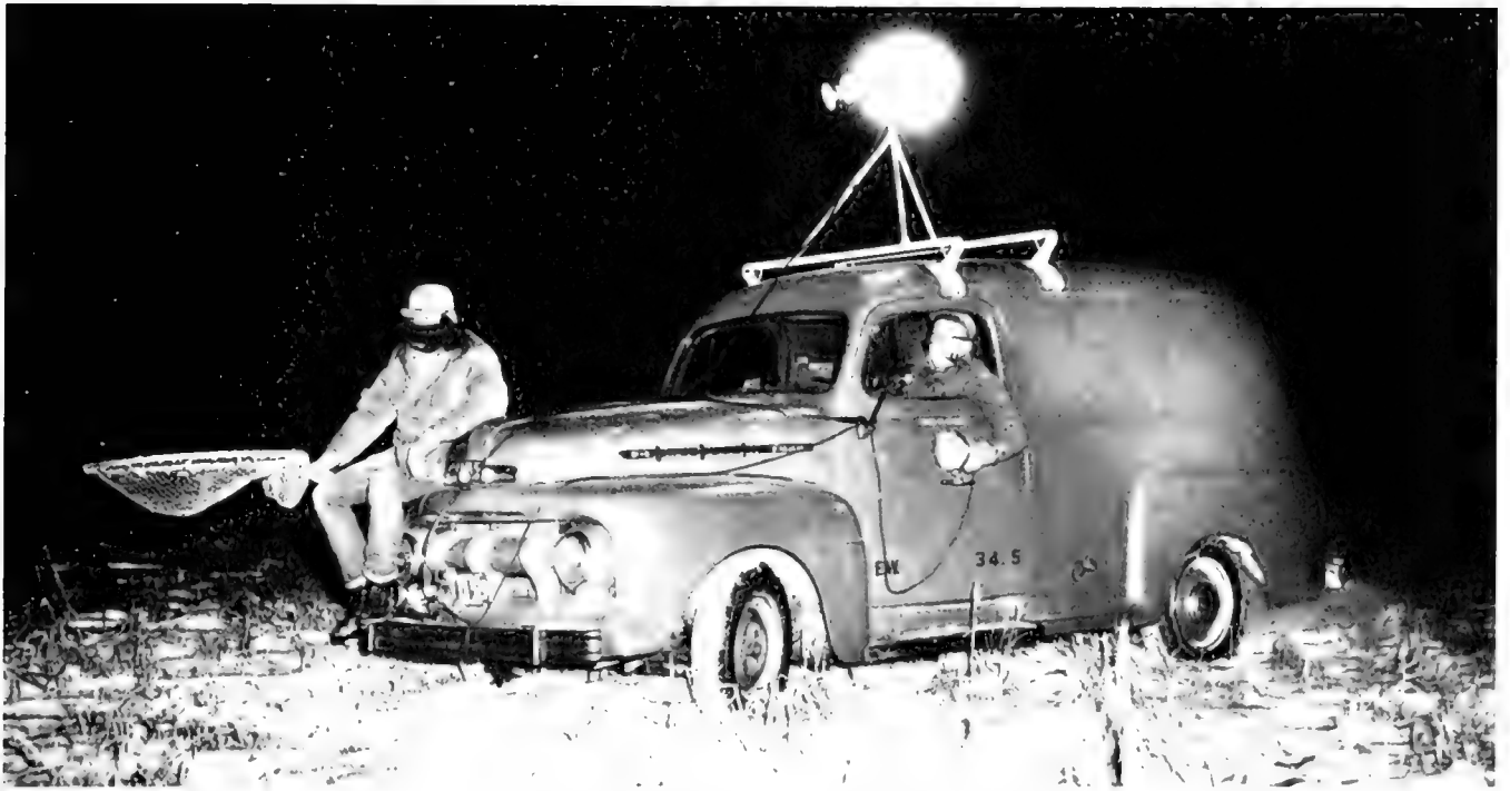
Fig. 5.—Night-lighting rig in operation in a grain stubble field. The electrical wiring system shown on this rig is an early design, less refined than the system that is described in this paper.
