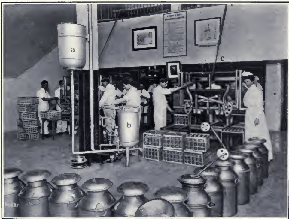
(a) MILK HEATER; (b) SEPARATOR; (c) BOTTLE FILLING MACHINE.
