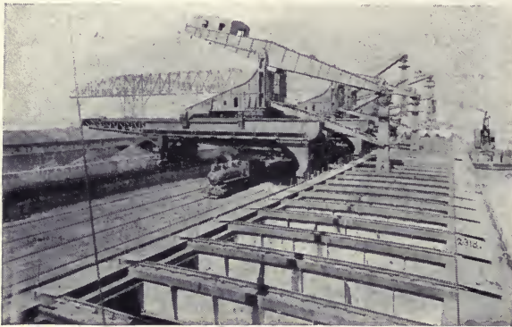
A GOOD VIEW OF THE HATCH SYSTEM OF MODERN ORE BOATS AND FOUR HULETT UNLOADERS AT WORK
