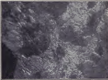
No. 23e. PEARLITE AT MAGNIFICATION OF 400 DIAMETERS
