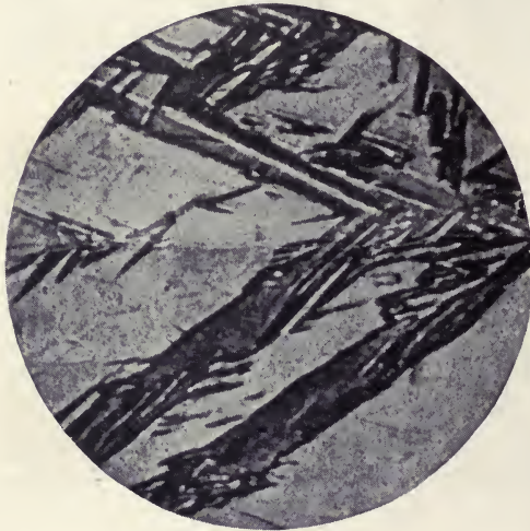
AUSTENITE (WHITE) AND MARTENSITE (DARK) MAGNIFIED 1,000 TIMES THEIR ACTUAL SIZE
