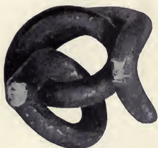
BAR IRON WILL STAND SEVERE BENDING EVEN AFTER IT HAS BEEN NICKED
