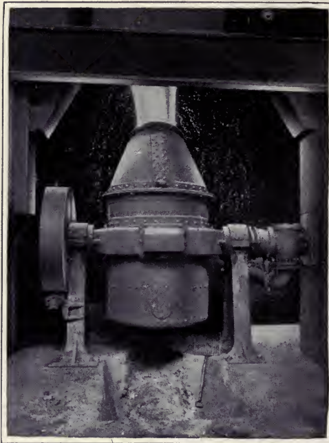
SMALL SIDE-BLOWN CONVERTER MAKING STEEL FOR CASTINGS
