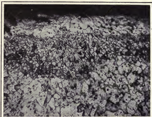
MALLEABLE CAST IRON IN WHICH PRACTICALLY ALL OF THE CARBON HAS BEEN REMOVED BY REAUMUR PROCESS ANNEALING
