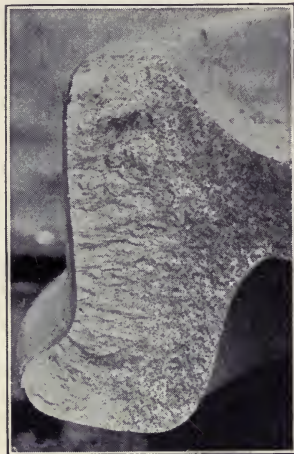
SECTION OF CHILLED CAR WHEEL Showing white iron rim.
