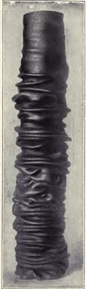
SHELBY SEAMLESS STEEL TUBING CRUSHED ENDWISE
