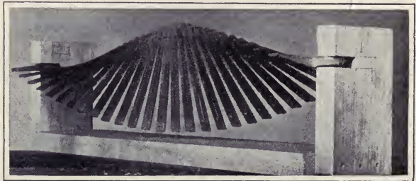
BECAUSE OF ITS ABILITY TO WITHSTAND BENDING AND 180- DEGREE TWISTS IT IS OFTEN JOCULARLY REFERRED TO AS THE "RUBBER CASTING." (FIG. C)
