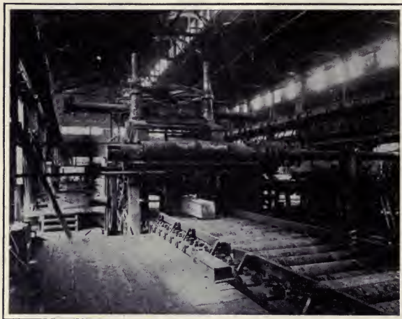
INGOT IN THE ROLLS
