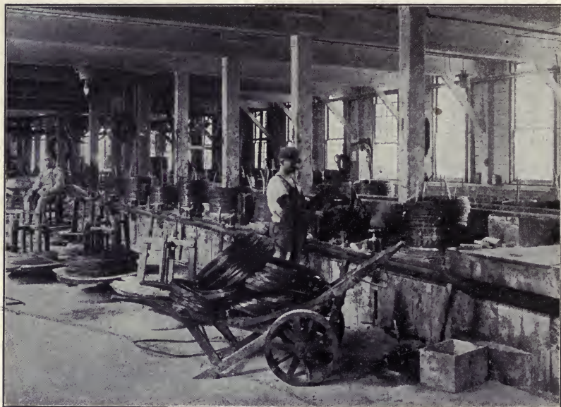
THE DRAWING OF WIRE
