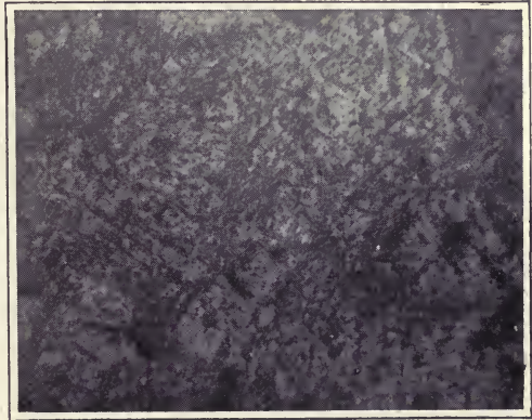
LOW CARBON TOOL STEEL (.50 PER CENT C) HARDENED (Magnification 100 diameters)
