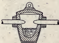
FIRST EXPERIMENTAL ARC ELECTRIC FURNACES PATENTED BY SIR WILLIAM SIEMENS IN 1879
