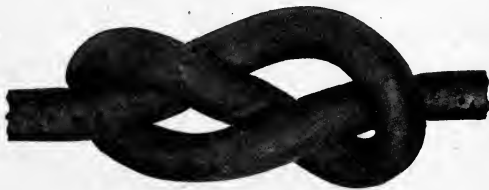
BOWKNOT MADE FROM PIECE OF STEEL PIPE
