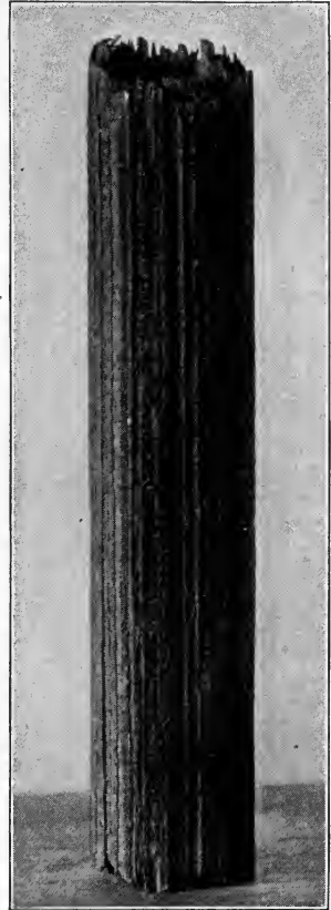
PICKLING IN WEAK ACID EX- POSES THE "FIBERS" OF WROUGHT IRON
