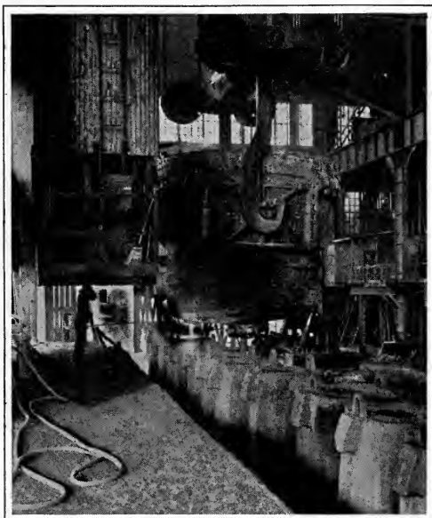
TEEMING THE STEEL INTO INGOT MOLDS
