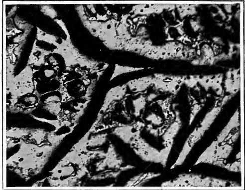
NO. 30. VERY SOFT CAST IRON. NOTE LARGE GRAPHITE FLAKES
