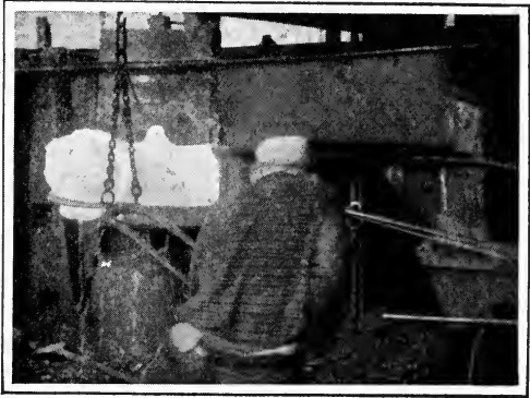
DRAWING ONE OF THE BALLS FROM THE FURNACE
