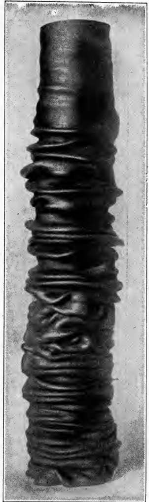
SHELBY SEAMLESS STEEL TUBING CRUSHED ENDWISE
