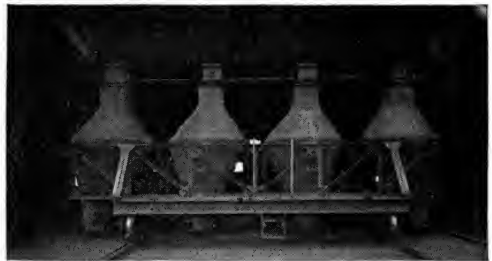
LORRY FOR CHARGING COAL INTO OVENS
