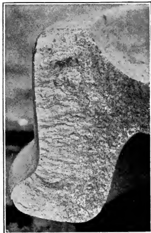
SECTION OF CHILLED CAR WHEEL
