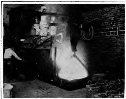
A GRONWALL-DIXON 5-TON ELECTRIC FURNACE TAPPING
