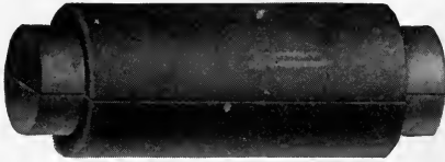
SPLIT PATTERN OF WOOD, SURFACE-COATED WITH SHELLAC VARNISH
