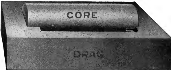
DRAG WITH CORE IN PLACE AND COPE, OR TOP HALF OF MOLD READY TO CLOSE
