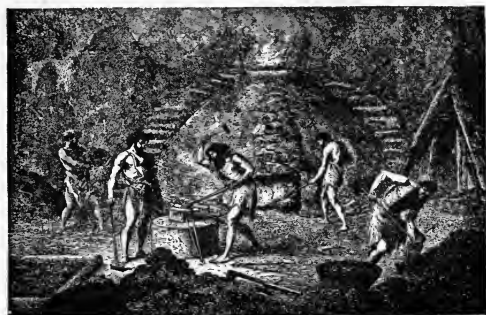
PRIMITIVE FURNACE FOR SMELTING IRON
