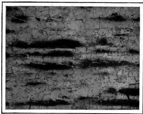
No. 1d. SECTION OF WROUGHT IRON CUT LENGTHWISE OF THE BAR. BLACK PATCHES AND FILAMENTS ARE "SLAG" OR "CINDER"
