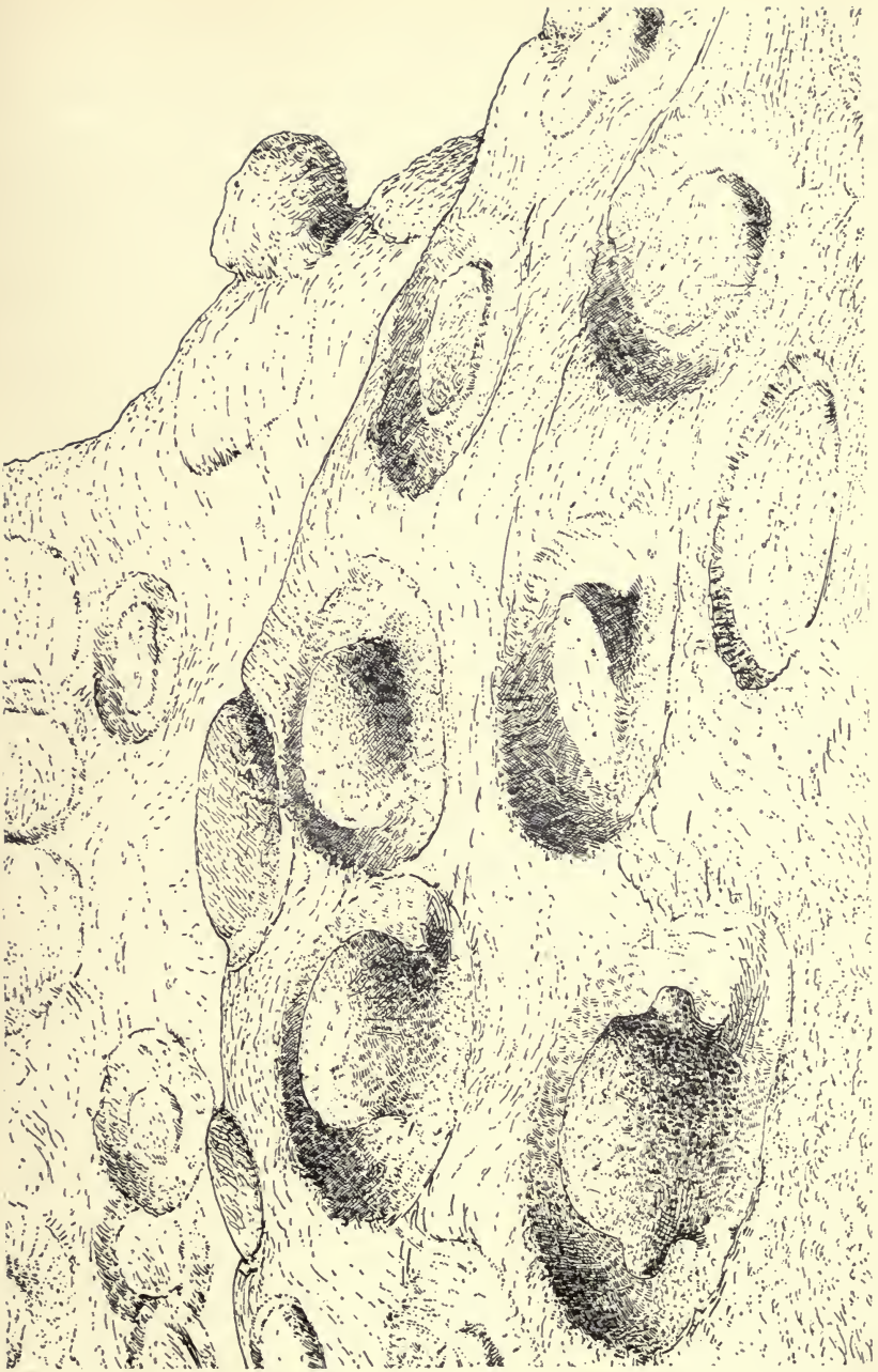
AMERICAN METHOD OF MINING STEATITE FOR UTENSILS
