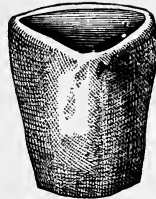
3. Hessian sand crucibles, round and tri- angular. (Fig. 8.)
