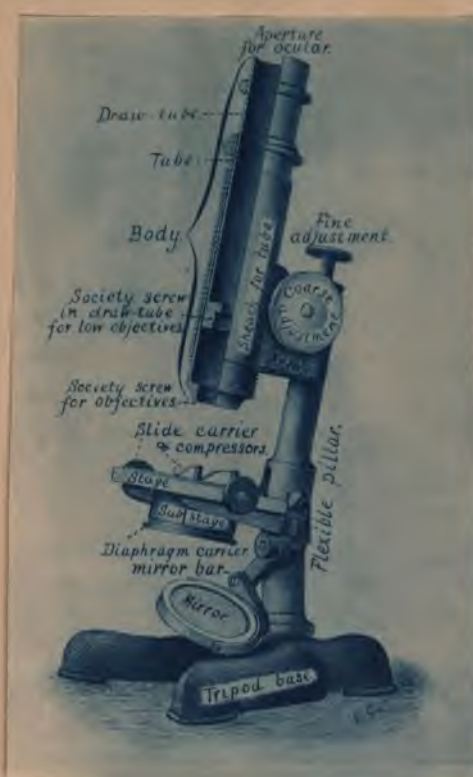
FIG. 3.—Stand of a Laboratory Compound Microscope with the parts named. A section has been removed from the body to show the position of the screw for the objective in the lower end of the body, and of the draw-tube.
