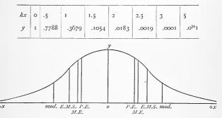
The ordinate represents the frequency of an error, the magnitude of which is represented by the corresponding abscissa. The curve is symmetrical about the *y*-axis, and shows points of inflection at
