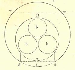
are also connected by suitable water pipes at the ends, both with each other, and with the water chamber of the large boiler, which completely encloses them, except at the ends. Being entirely below water level, they are by these connexions kept constantly filled with water. These interior boilers are suspended, and kept in place by rods coming down from an iron cross beam, resting on the wall of the furnace, beyond the ends of the large shells Aand B.
