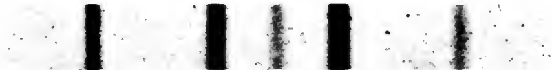
A photographic record of the mass spectrum of germanium, showing the isotopes of mass numbers 70, 72, 73, 74, and 76.
