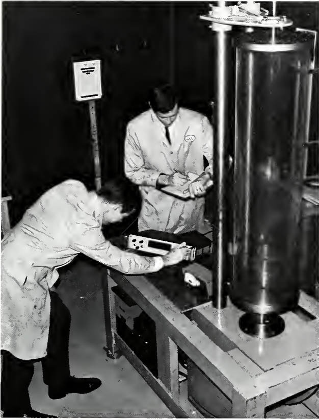
Checking the results of an experiment, graduate students operate the new rotating fluid demonstration unit for a research project.
