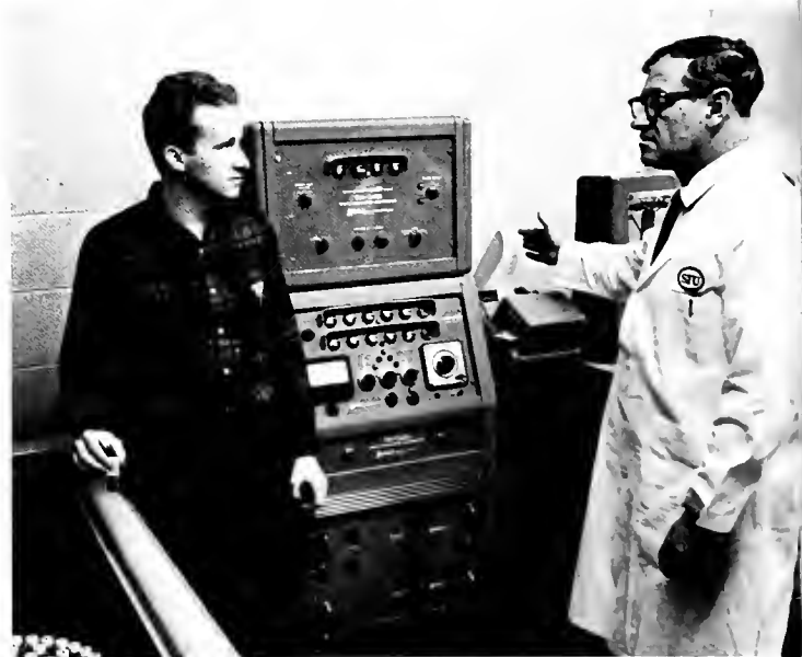
Maurice Ogur, director of the Biological Research Laboratory, demonstrates to Ramon Tait, the operation of a liquid scintillation spectrometer, a machine which counts radioactive isotopes in samples of yeast cultures investigated for structure and internal processes.
