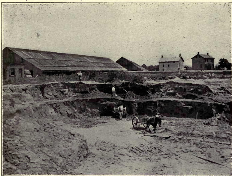
FIG. 1.—Digging clay by means of open pits. At the top of the bank, in the background, a workman is driving a wedge into the clay in order to break it off. The clay is hauled to the yards in carts. (After Ries, N. J. Geol. Surv., Fin. Rept., VI, p. 35, 1904.)
