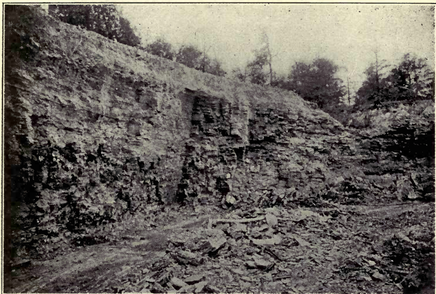
FIG. 1.—Carboniferous shale for paving-blocks near Veedersburg, Ind. (After Blatchley, 29th Ann. Rep., Ind. Dept. Geol. and Nat. Res., p. 80.)
