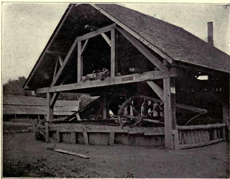
FIG. 2.—Ring-pit for mixing clays. (After H. Ries, N. Y. State Museum, Bull. 35, p. 659, 1900.)
