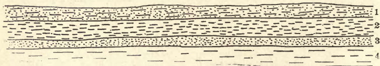
FIG. 8.—Section of horizontal strata, with only the top one exposed at the surface.
