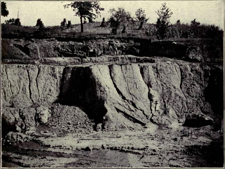
FIG. 1.—Deposit of calcareous glacial clay, Ionia, Mich. (After H. Ries, Mich. Geol. Surv., VIII, Pt. I, p. 52, 1900.)
