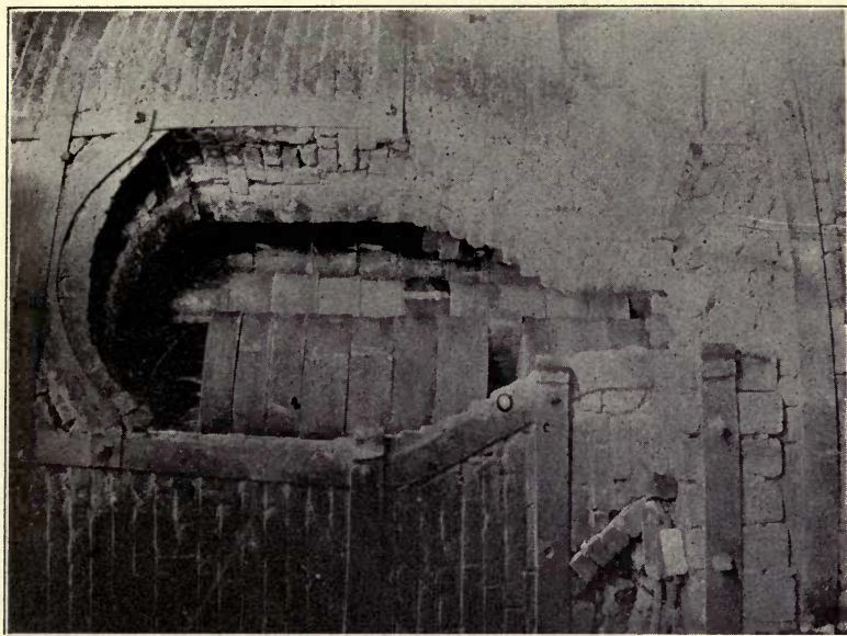
FIG. 2.—Partial interior view of a pottery-kiln, showing saggars in which white wares are burned. (Photo by H. Ries.)
