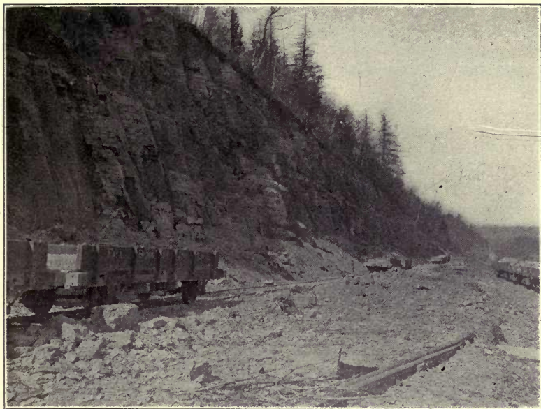
FIG. 1.—Bank of Chemung shale used for brick, Corning, N. Y. (After H. Ries, N. Y. State Mus., Bull. 35, p. 838, 1900.)
