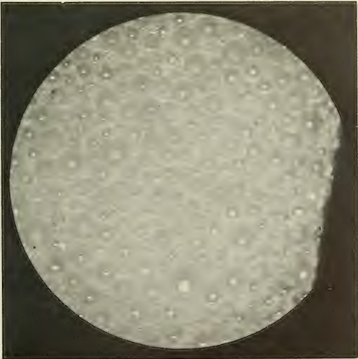
Syntactic foam, one of the low-density materials being developed for use as auxiliary buoyancy for deep-submergence vehicles. It is composed of hollow glass microspheres embedded in a plastic matrix and has a density of 40 to 46 lb/ft 3 .
