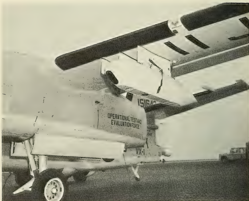
A radiation thermometer mounted on the wing of a S2E aircraft permits measurement of the sea-surface temperature over a large area in a short time period.
