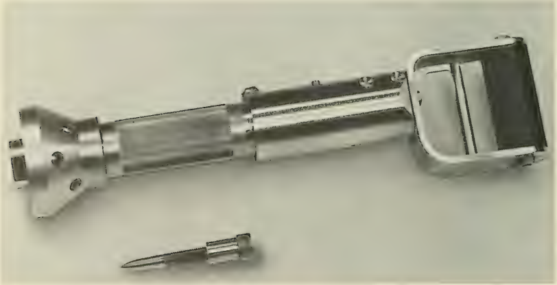
Large-velocity powered stud gun. Capable of operating to 1000 ft, this gun can drive solid steel studs into 1-1/8-in. thick mild steel plate.
