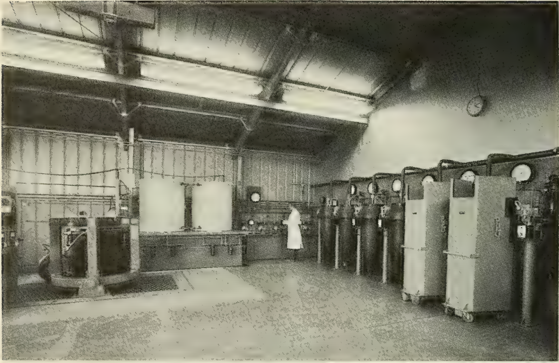
The Deep Ocean Simulation Laboratory at NCEL, showing six 9-in.-ID pressure vessels and one 18-in.-ID pressure vessel used to simulate the deep-ocean environment. Tanks in the background are for sea water storage.
