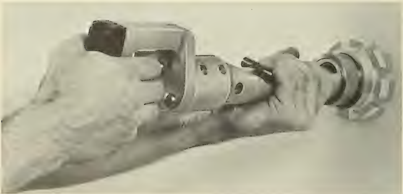
Small-velocity powered stud gun, a lightweight, underwater hand-held tool used to punch holes in steel plate or attach studs to metal objects underwater
