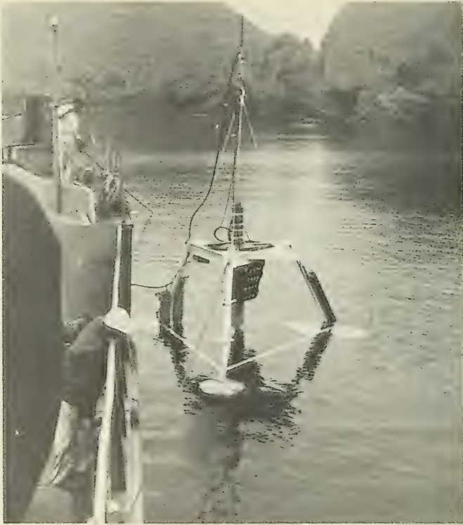
The NCEL "Padlock" anchor being lowered into the water. This anchor is designed to support a load in any direction and will have a depth capability of 6000 ft.
