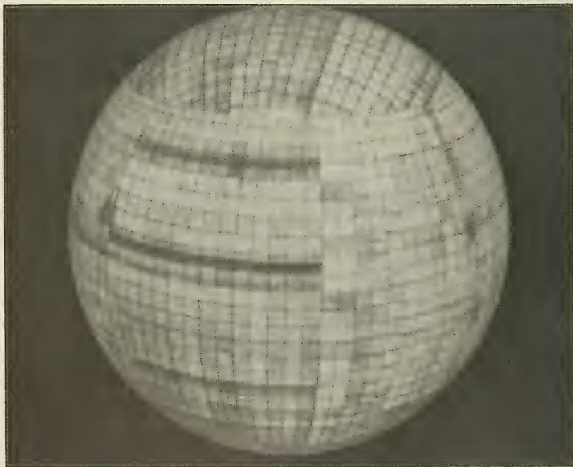
Fiberglass reinforced plastic sphere, a recently developed low-density material for use as auxiliary buoyancy in deep-submergence vehicles
