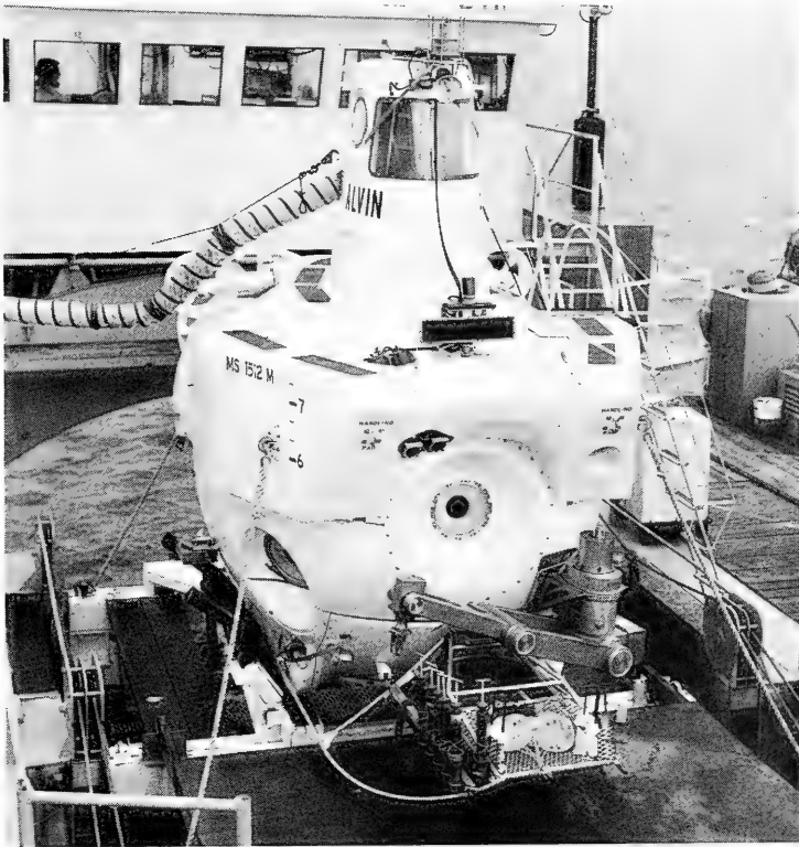
Deep-submergence vehicle ALVIN rigged for a science mission. Drop-able working tray is shown in place, with mechanical manipulator and bottom working tools for a geologic dive.
