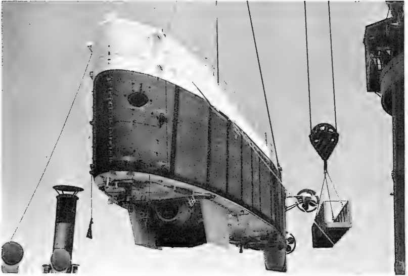
U. S. Navy TRIESTE II, successor to TRIESTE I, a bathyscaph with modern navigation and control equipment, TV cameras, lights, and mechanical arm. TRIESTE II located and photographed portions of the THRESHER in 1964.
