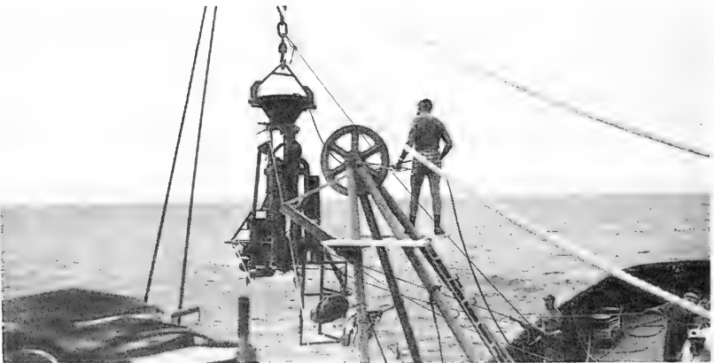
Submerged Object Recovery Device (SORD). SORD can be used in deep-ocean recovery and salvage. Objects are picked up with a snare manipulated from the surface by personnel using closed-circuit TV for direction.
