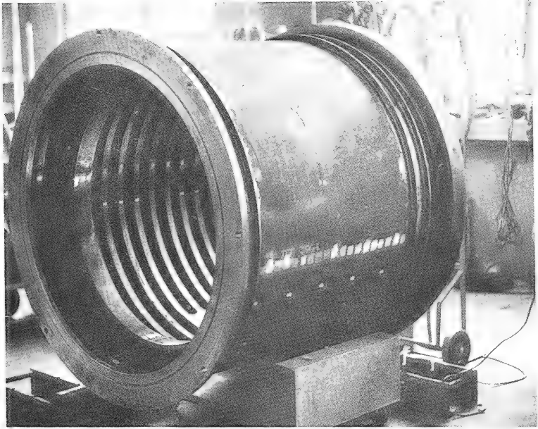
HY 130/150 steel cylinder model. This model was used to study fabrication and the structural performance of welded HY-130/150 steel, the hull material to be used in the Navy's Deep Submergence Rescue Vehicle (DSRV).
